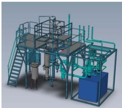
*3D view of the complete BioZEG plant including SER reactor system (left) and SOFC module (right)*
