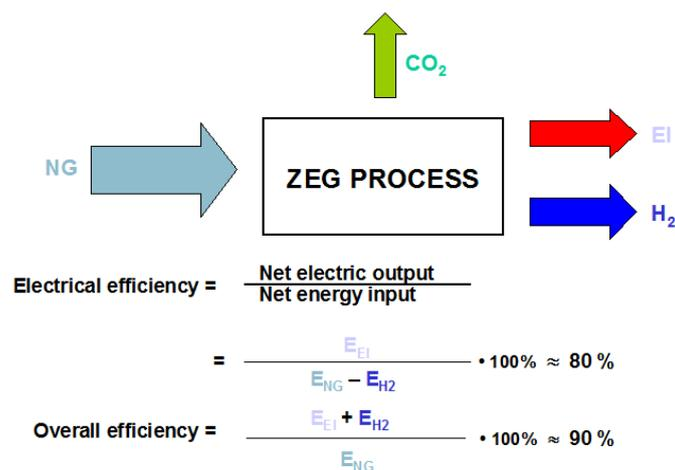
Figure 2 Energy efficiency of ZEG-concept
