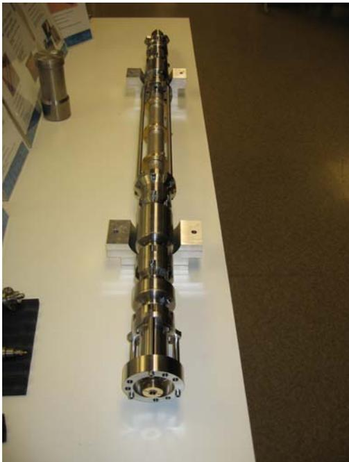
Figure 3.7 High temperature NIR gas characterization measurement cell
