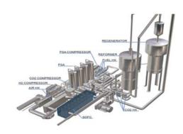
The**BioZEG**-project (completed in 2013) represented a significant up scaling from 2kW to 50kW and introduced heat integration between SOFC and the fluidized bed regenerator in the SER reactor system. The **ZEG**<sub>400</sub> project will also include a dedicated heat-transfer loop and recycling of hydrogen for further efficiency optimization. Main issues addressed in a test program of a 400kW scale pilot will be:
