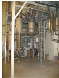
30kW<sub>H<sub>2</sub></sub> SER reactor system, by IFE
