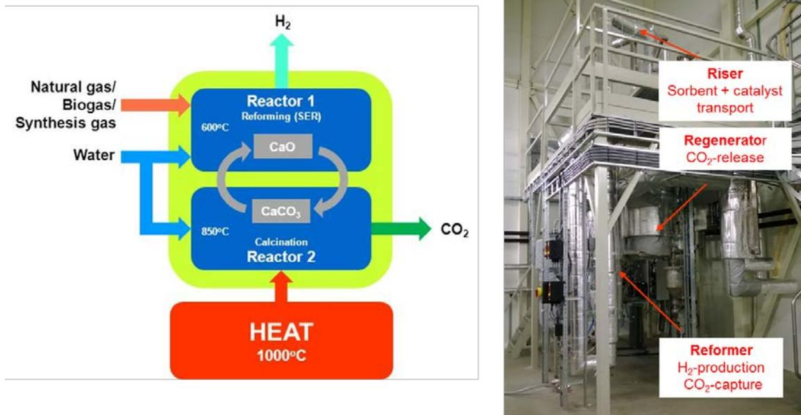
Figure 5 – Sorption enhanced steam methane reforming (SESMR) process principle (left) and bubbling fluidized bed (DBFB) pilot plant (right)
