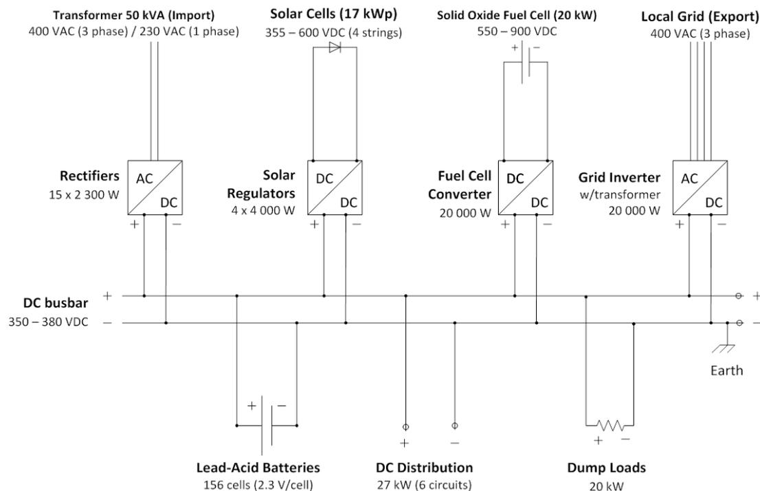
Figure 7 – PV and fuel cell power system
