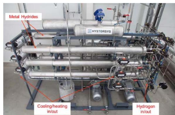
Figure 3 – Metal hydride hydrogen compressor
