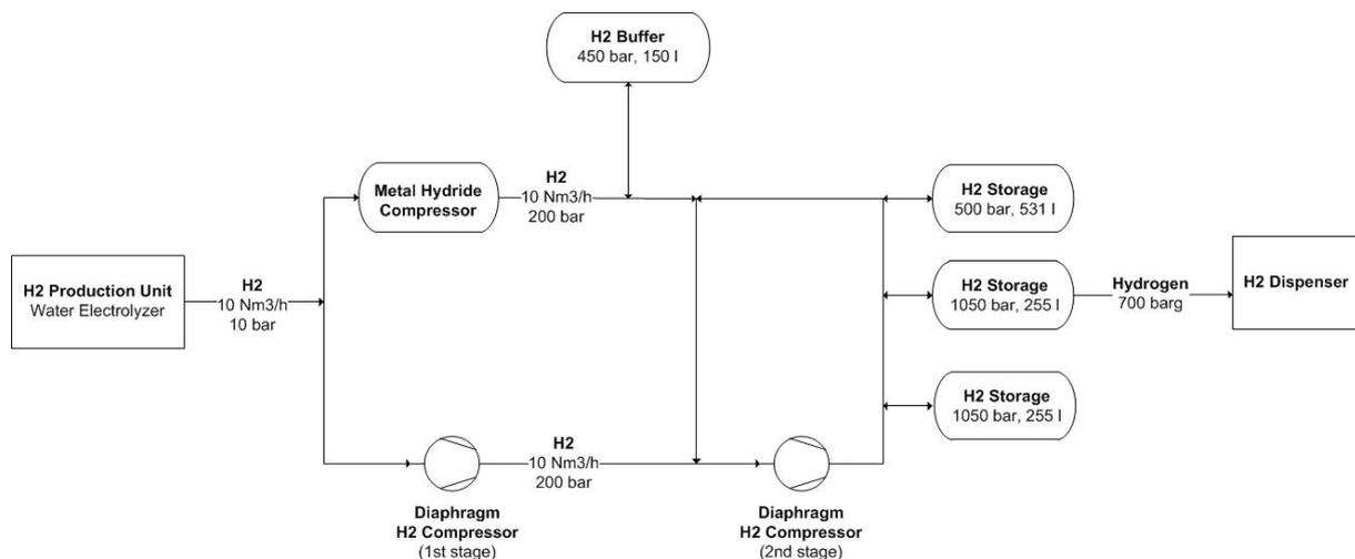
Figure 4 – Process flow diagram of hydrogen compression system with metal hydrides
