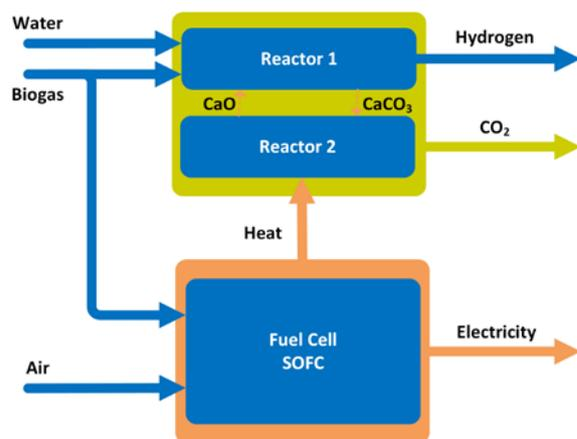
Figure 6 – The BioZEG-concept: SESMR and SOFC system integration
