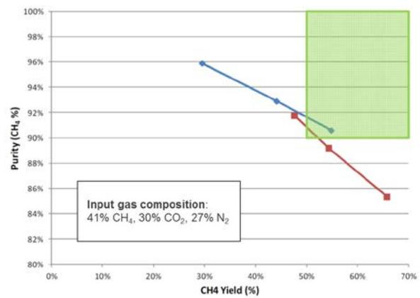
Figure 8 – Summary of small-scale PSA laboratory tests performed at HyGear [6]. Green area: Multiple tests performed at fixed operating conditions (adsorption pressure, cycle time, etc). Blue and red curves: Tests with different control settings.
